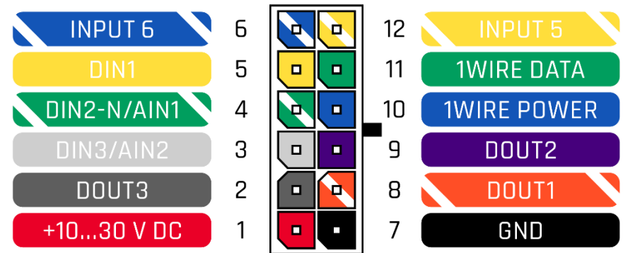
Figure 2 FMB130 2x6 socket pinout
